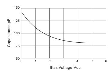
Capacitance vs. Biasing Voltage@1MHz
