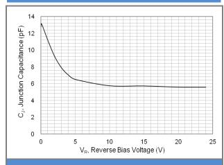
Fig.1 Typical Junction Capacitance(24V)
