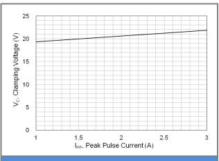
Fig.4 Typical Peak Clamping Voltage(8/20μs)(15V)
