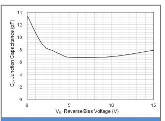
Fig.2 Typical Junction Capacitance(15V)
