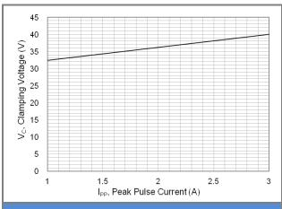
Fig.3 Typical Peak Clamping Voltage(8/20µs)(24V)
