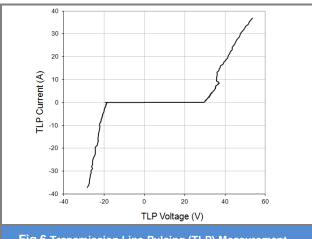
Fig.6 Transmission Line Pulsing (TLP) Measurement
