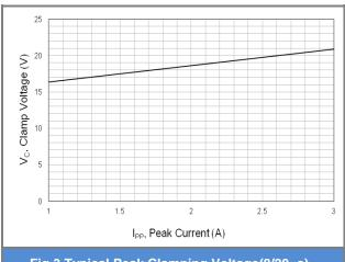
Fig.3 Typical Peak Clamping Voltage(8/20μs)
