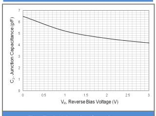
**Fig.1 Typical Junction Capacitance**
