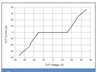
Fig.2 Transmission Line Pulsing (TLP) Measurement
