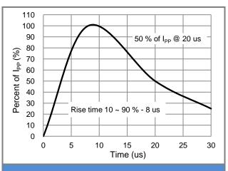
Fig.2 Pulse Waveform
