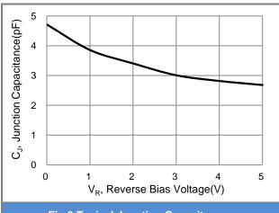
Fig.3 Typical Junction Capacitance
