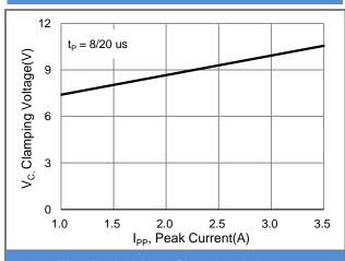
Fig.1 Typical Peak Clamping Voltage
