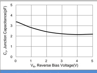
Fig.3 Typical Junction Capacitance
