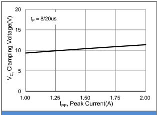
Fig.1 Typical Peak Clamping Voltage
