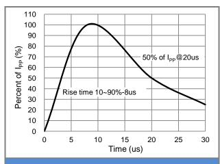
Fig.2 Pulse Waveform
