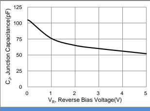
Fig.3 Typical Junction Capacitance
