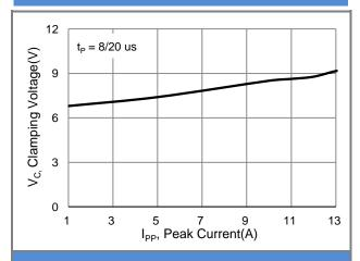
Fig.1 Typical Peak Clamping Voltage
