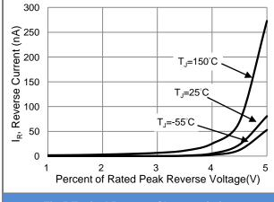
**Fig.5 Typical Reverse Characteristics**
