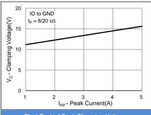
Fig.1 Typical Peak Clamping Voltage
