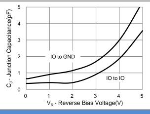
Fig.3 Typical Junction Capacitance
