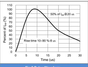
Fig.2 Pulse Waveform
