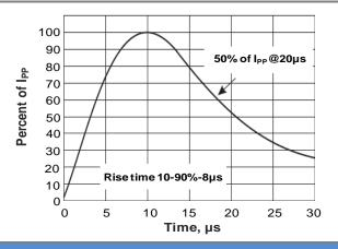
Fig.4 8/20µs Pulse Waveform
