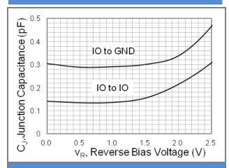
Fig.1 Typical Junction Capacitance
