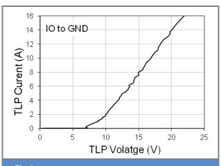
Fig.2 Transmission Line Pulsing (TLP) Measurement
