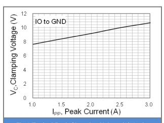
Fig.3 Typical Peak Clamping Voltage(8/20µs)
