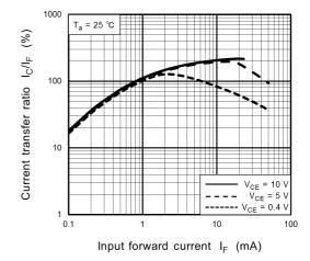
Fig. 11.12 I<sub>C</sub>/I<sub>F</sub> - I<sub>F</sub>
