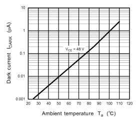
Fig. 11.9 I<sub>DARK</sub> - T<sub>a</sub>
