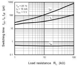
Fig. 11.14 Switching Time - R<sub>L</sub>
