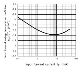
Fig. 11.5  $\Delta V_F/\Delta T_a - I_F$
