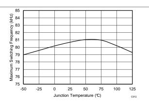
Figure 8. Maximum Switching Frequency vs Junction Temperature
