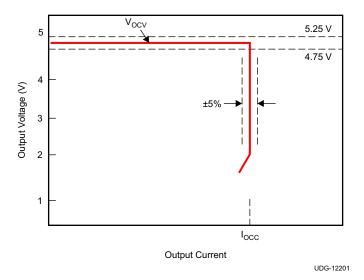
Figure 17. Typical Target Output V-I Characteristic
