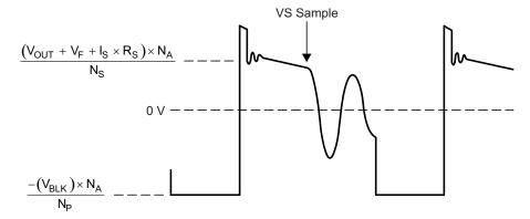
Figure 13. Auxiliary Winding Voltage
