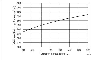
Figure 7. Minimum Switching Frequency vs Junction Temperature
