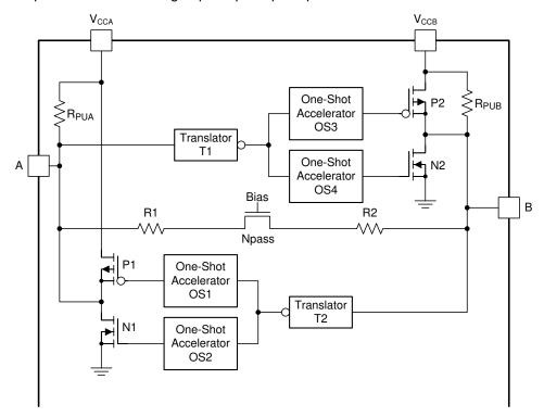
Figure 12. Architecture of a TXS0108E-Q1 Cell
