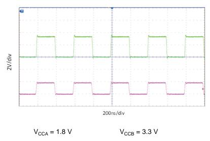
Figure 14. Level-Translation of a 2.5-MHz Signal
