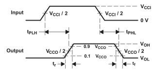
Figure 9. Propagation Delay Times
