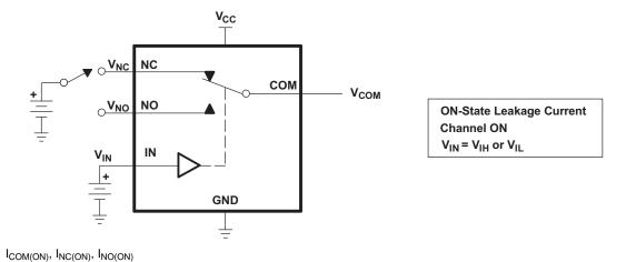
Figure 7. ON-State Leakage Current
