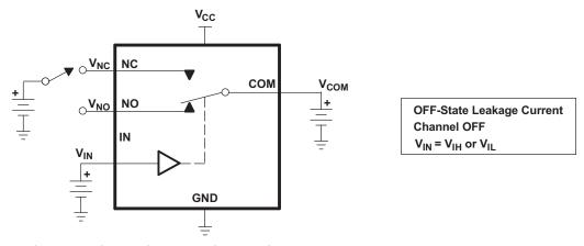
$I_{NC(OFF)},\ I_{NC(PWROFF)},\ I_{NO(OFF)},\ I_{NO(PWROFF)},\ I_{COM(OFF)},\ I_{COM(PWROFF)}$
