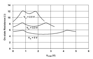
Figure 17. ron vs V<sub>COM</sub>
