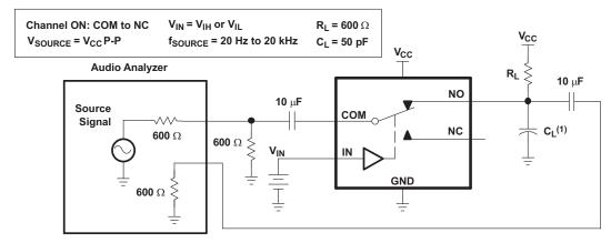
(1)  $C_L$  includes probe and jig capacitance.
