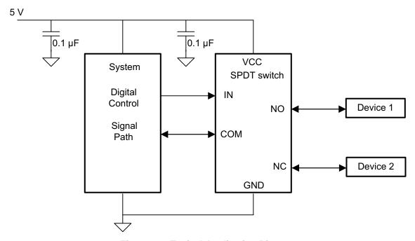
Figure 16. Typical Application Diagram
