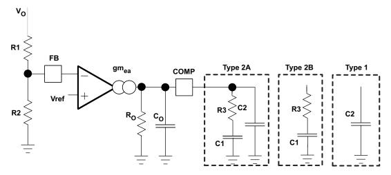
Figure 32. Types of Frequency Compensation
