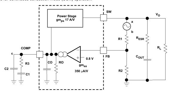
Figure 30. Small Signal Model for Loop Response
