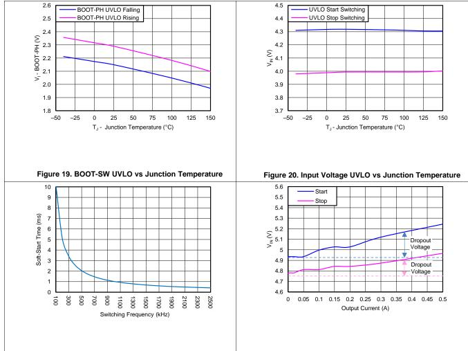
Figure 21. Soft-Start Time vs Switching Frequency
