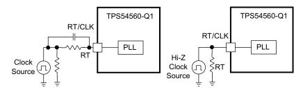
Figure 26. Synchronizing to a System Clock
