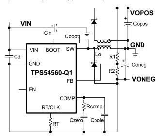
Figure 35. TPS54560-Q1 Split Rail Power Supply based on the SLVA369 Application Note
