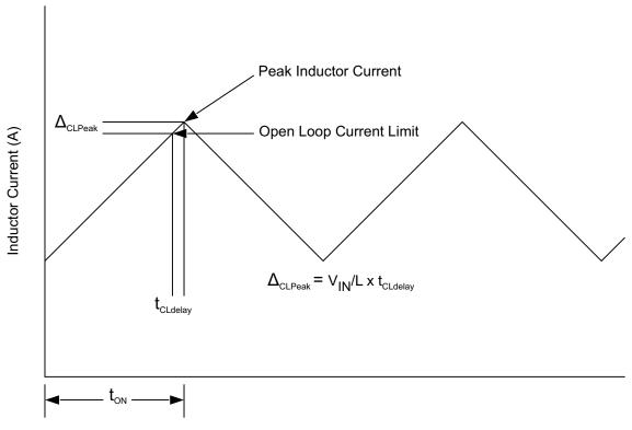
Figure 25. Current Limit Delay
