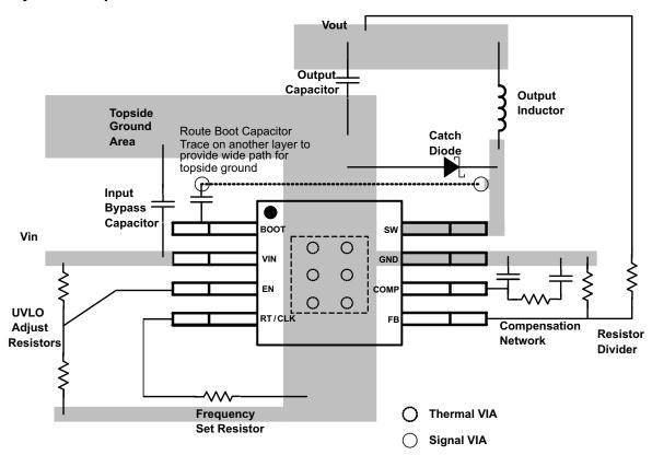
Figure 57. PCB Layout Example
