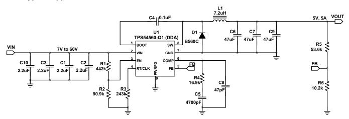
Figure 36. 5 V Output TPS54560-Q1 Design Example
