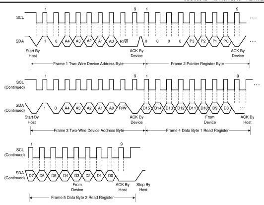
Figure 9-5. Two-Wire Timing Diagram for Read Word Format
