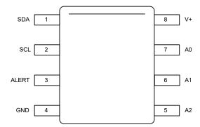
Figure 7-1. D Package 8-Pin SOIC Top View
