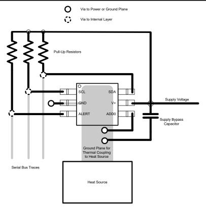
Figure 12-4. Layout Example (DRL Package)
