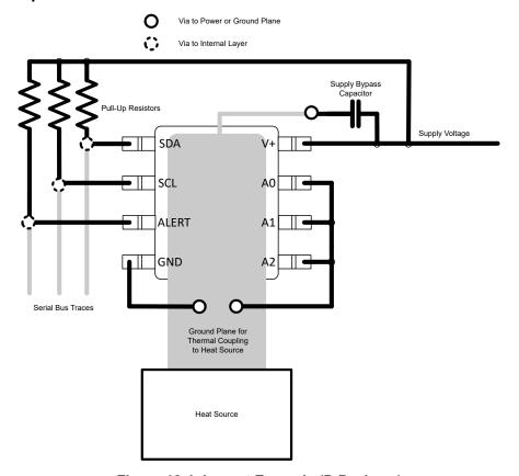
Figure 12-1. Layout Example (D Package)
