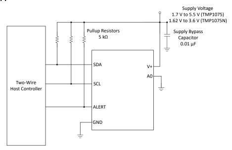
Figure 10-1. Typical Connections
