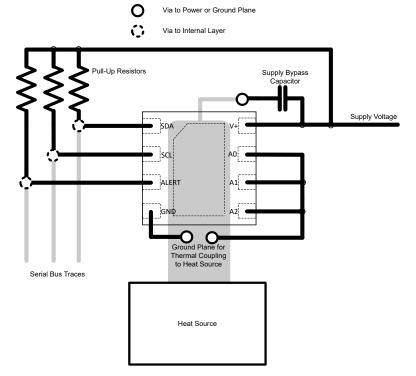
Figure 12-3. Layout Example (DSG Package)
