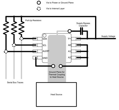
Figure 12-2. Layout Example (DGK Package)
