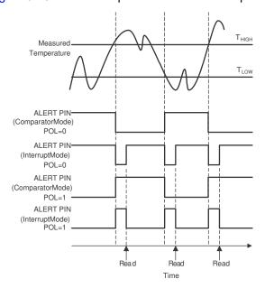
Figure 9-10. Output Transfer Function Diagrams
