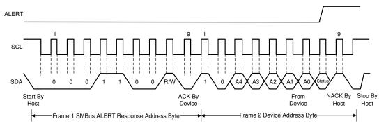
Figure 9-8. Timing Diagram for SMBus Alert
