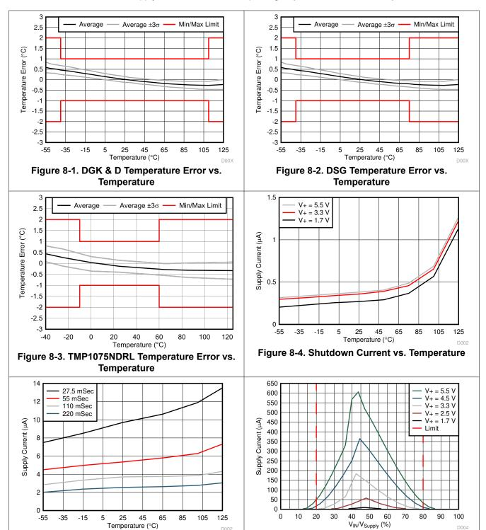
Figure 8-5. Average Current vs. Conversion Rates and Temperature
