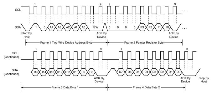
Figure 9-3. Two-Wire Timing Diagram for Write Word Format
