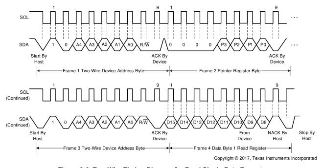
Figure 9-6. Two-Wire Timing Diagram for Read Single Byte Format
