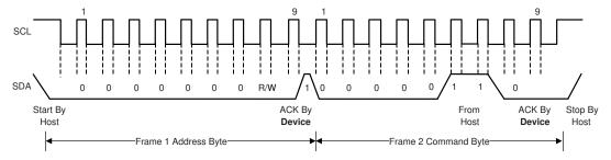
Figure 9-7. General-Call Reset Command Timing Diagram
