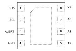
Figure 7-2. DGK Package 8-Pin VSSOP Top View
