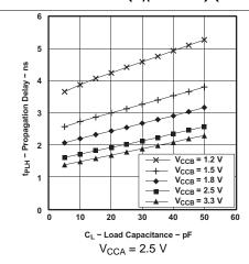
Figure 7. Typical Propagation Delay t<sub>PLH</sub> (A to B) vs Load Capacitance
