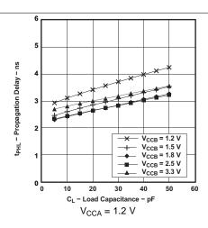
Figure 2. Typical Propagation Delay t<sub>PHL</sub> (A to B) vs Load Capacitance
