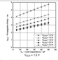
Figure 1. Typical Propagation Delay t<sub>PLH</sub> (A to B) vs Load Capacitance
