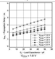
Figure 6. Typical Propagation Delay t<sub>PHL</sub> (A to B) vs Load Capacitance
