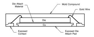
Figure 27. Internal WSON Connection
