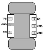
Figure 26. 6-Lead WSON PCB Dog Bone Layout
