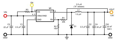
Figure 15. Typical Application Schematic
