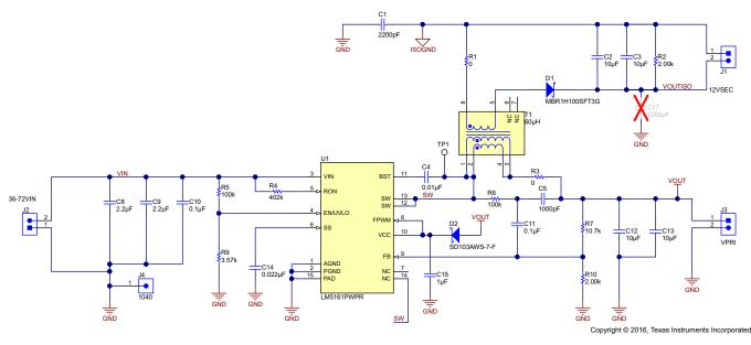
Figure 34. 12-V, 10-W Fly-Buck Schematic
