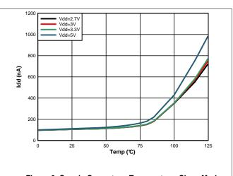
Figure 8. Supply Current vs. Supply Voltage, Sleep Mode Figure 9. Supply Current vs. Temperature, Sleep Mode
