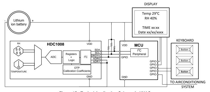
Figure 15. Typical Application Schematic HVAC
