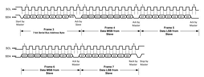
Figure 14. Read Humidity and Temperature Measurement (Data Ready)
