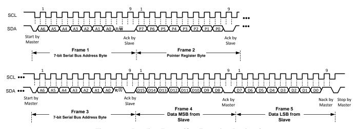
Figure 11. Reading Frame (Configuration Register)
