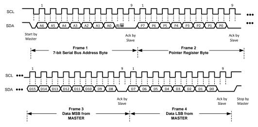
Figure 10. Writing Frame (Configuration Register)
