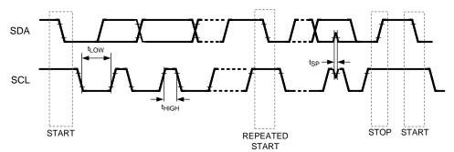
Figure 1. I<sup>2</sup>C Timing
