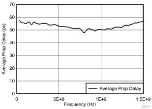
Figure 1. Average Propagation Delay vs Frequency
