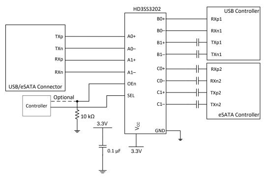
Figure 15. eSATA and USB 3.1 Combo Connector
