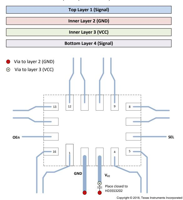
Figure 17. HD3SS3202 Basic Layout Example
