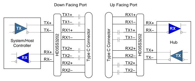
Figure 8. AC Coupling Capacitors for USB Type C
