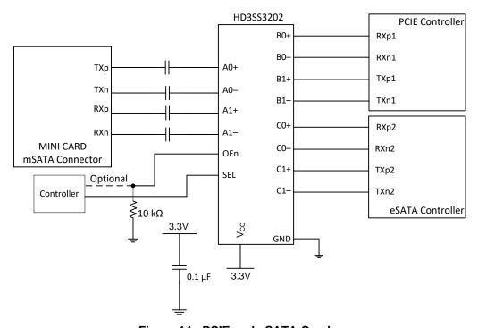
Figure 14. PCIE and eSATA Combo
