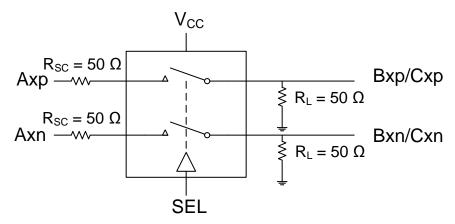
Figure 2. Test Setup
