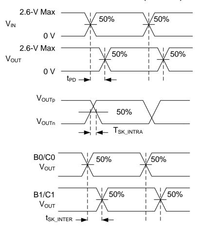
Figure 4. Timing Diagrams and Test Setup
