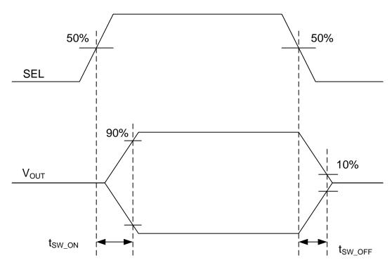
Figure 3. Switch On and Off Timing Diagram
