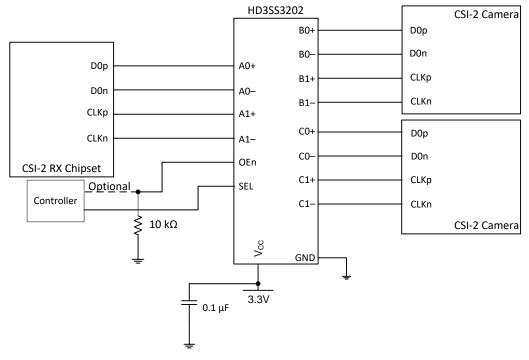
Figure 16. CSI Camera Array
