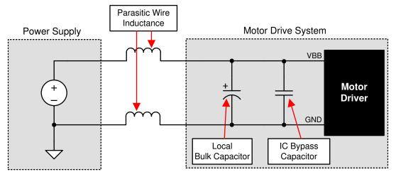
Figure 9-1. System Supply Parasitics Example
