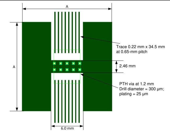
Figure 8-2. HTSSOP PCB model top layer
