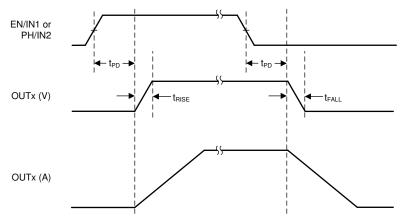
Figure 6-1. Timing Parameter Diagram
