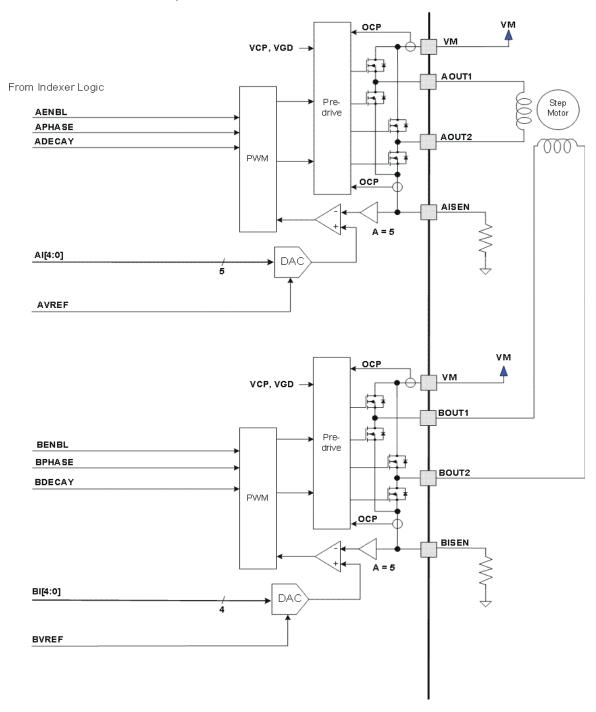
Figure 7-1. Motor Control Circuitry
