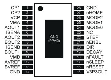
Figure 5-1. PWP Package 28-Pin HTSSOP Top View
