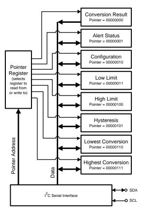
Figure 21. Register Structure
