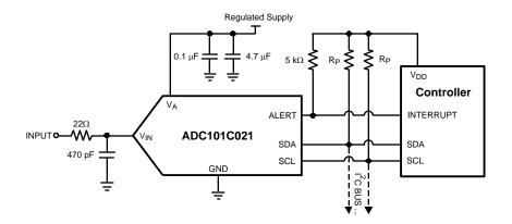
Figure 33. Typical Application Circuit
