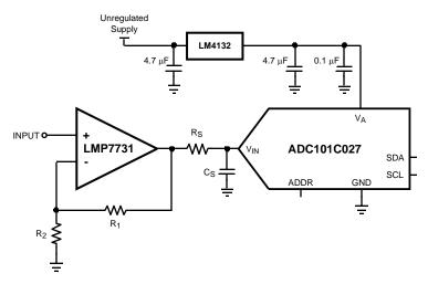
Figure 34. Buffered Input Circuit
