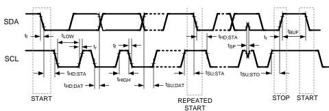
Figure 1. Serial Timing Diagram
