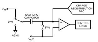
Figure 17. ADC101C021 in Track Mode
