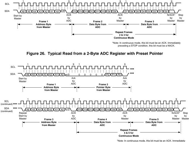
\*Note: In continuous mode, this bit must be an ACK. Immediately preceding a STOP condition, this bit must be a NACK.
