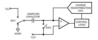
Figure 18. ADC101C021 in Hold Mode
