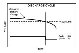
Figure 37. Discharge Cycle
