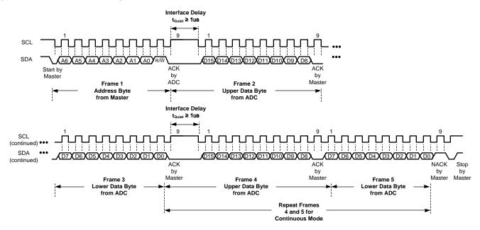
Figure 32. Reading in Quiet Interface Mode
