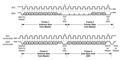
Figure 29. Typical Pointer Set Followed by Immediate Read of a 1-Byte ADC Register
