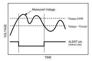
Figure 24. Alert condition cleared when measured voltage crosses V<sub>HIGH</sub> - V<sub>HYST</sub>
