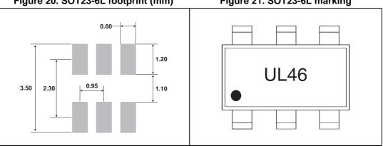
Figure 21. SOT23-6L marking
