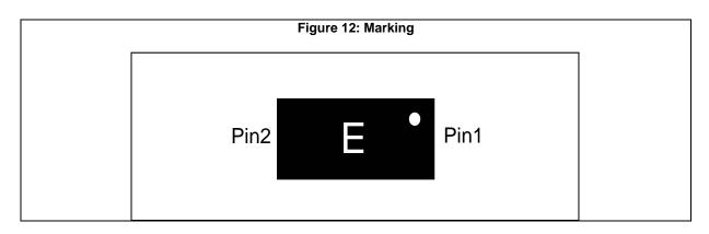
Product marking may be rotated by multiples of 90° for assembly plant differentiation. In no case should this product marking be used to orient the component for its placement on a PCB. Only pin 1 mark is to be used for this purpose.
