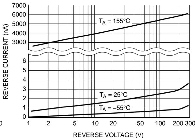
Figure 3. Reverse Leakage
