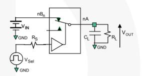
Figure 6. Test Circuit Load
