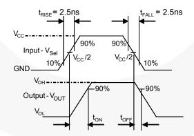
Figure 7. Turn-On / Turn-Off Waveforms
