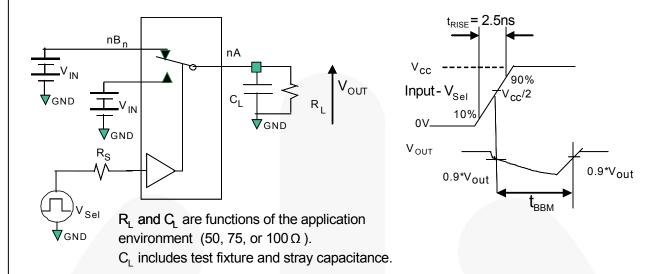
Figure 8. Break-Before-Make Interval Timing
