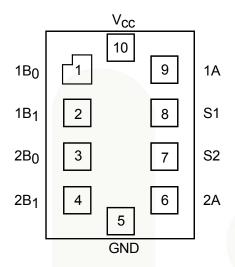
Figure 2. 10-Lead MicroPak™ (Top-Through View)
