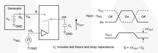
Figure 12. Charge Injection Test
