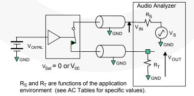
Figure 15. Total Harmonic Distortion
