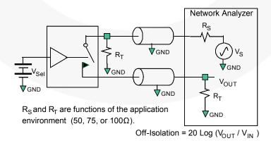
Figure 10. Channel Off Isolation
