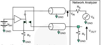
$R_S$  and  $R_T$  are functions of the application environment (50, 75, or 100 $\Omega$ ). CROSSTALK = 20 Log ( $V_{OUT}/V_{IN}$ )
