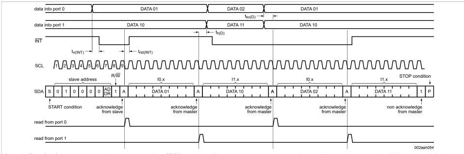
**Remark:** Transfer of data can be stopped at any moment by a STOP condition. When this occurs, data present at the latest acknowledge phase is valid (output mode). It is assumed that the command byte has previously been set to '00' (read input port register).
