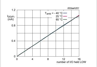
Figure 28. Supply current versus number of I/O held LOW
