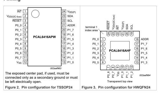
Low-voltage translating 16-bit I<sup>2</sup>C-bus/SMBus I/O expander with interrupt output, reset, and configuration registers
