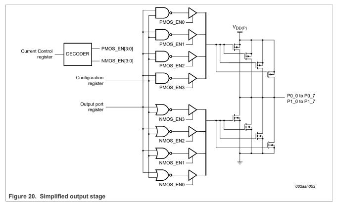
Reducing the current drive capability may be desirable to reduce system noise. When the output switches (transitions from H/L), there is a peak current that is a function of the output drive selection. This peak current runs through  $V_{DD}$  and  $V_{SS}$  package inductance
