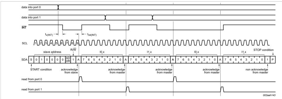
**Remark:** Transfer of data can be stopped at any moment by a STOP condition. When this occurs, data present at the latest acknowledge phase is valid (output mode). It is assumed that the command byte has previously been set to '00' (read input port register).
