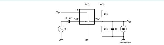
With  $f_i$  = 1 MHz adjust the switch input voltage for a 0 dBm level at the switch output, (0 dBm = 1 mW into 50  $\Omega$ ). Then increase the input  $f_i$  frequency until the dB meter reads -3 dB.
