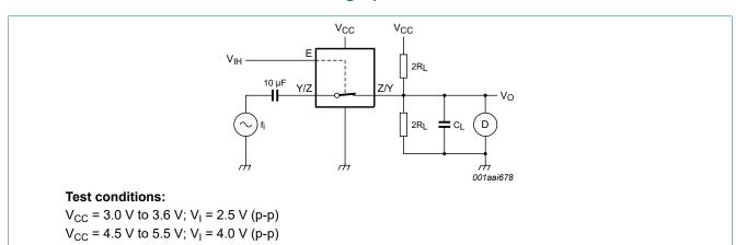
Fig. 11. Test circuit for measuring total harmonic distortion
