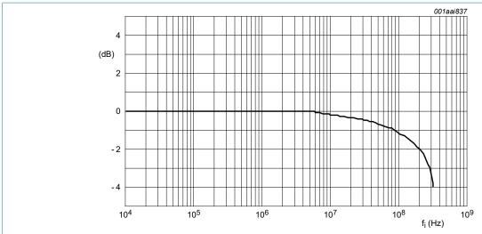
Test conditions:  $V_{CC}$  = 4.5 V; GND = 0 V;  $R_L$  = 50  $\Omega$ ;  $R_{SOURCE}$  = 1 k $\Omega$ .
