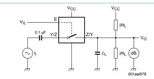
Adjust the switch input voltage for a 0 dBm level (0 dBm = 1 mW into 600  $\Omega$ ).
