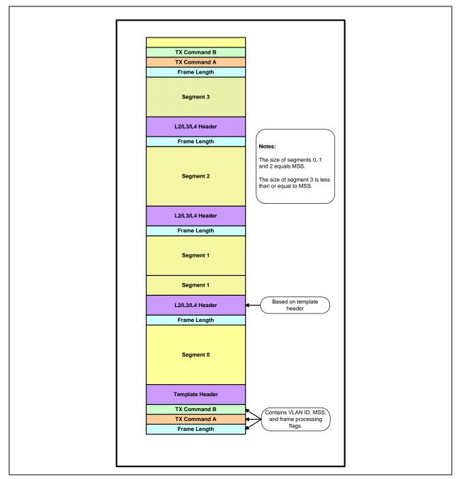
FIGURE 6-5: LSO TX FIFO FRAME STORAGE
