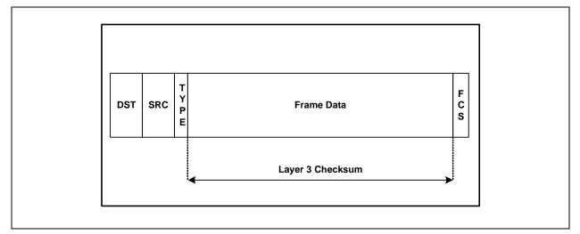
Consider the case where the frame is a 802.3 Ethernet frame with a VLAN tag. The RFE bypasses DA, SA, VLAN tag, SNAP header, and type fields. The calculation begins at the byte immediately following the type field. The calculation does not include the FCS.
