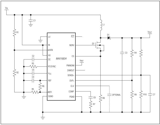
Figure 6. Boost DC-DC Converter
