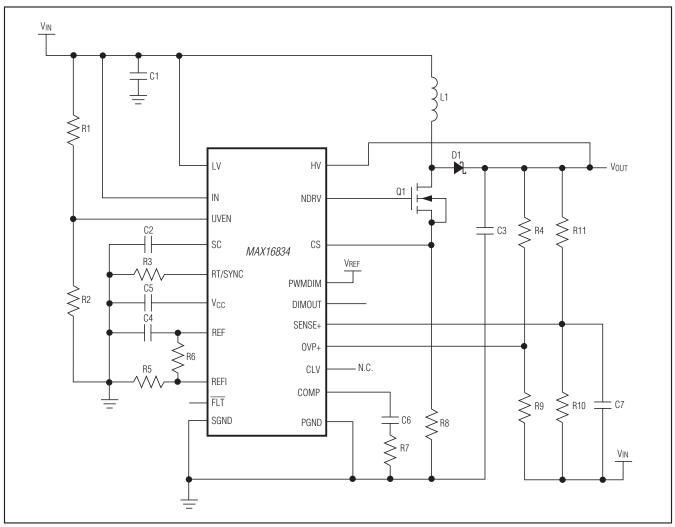
Figure 7. Boost-Buck DC-DC Converter
