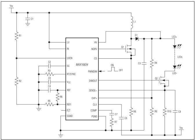
Figure 3. Boost-Buck LED Driver (V<sub>LED+</sub> < 28V)
