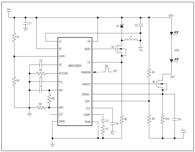
Figure 5. High-Side Buck LED Driver
