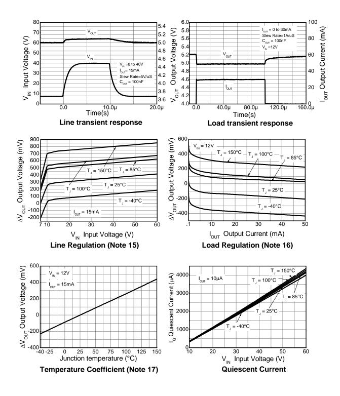
Notes: 15. Line Regulation  $\Delta V_{OUT} = V_{OUT} - V_{OUT} (@V_{IN} = 7V, I_{OUT} = 15mA, T_J = +25^{\circ}C)$ . 16. Load Regulation  $\Delta V_{OUT} = V_{OUT} - V_{OUT} (@V_{IN} = 12V, I_{OUT} = 0.1mA, T_J = +25^{\circ}C)$ . 17. Temperature Coefficient  $\Delta V_{OUT} = V_{OUT} - V_{OUT} (@V_{IN} = 12V, I_{OUT} = 15mA, T_J = +25^{\circ}C)$ .
