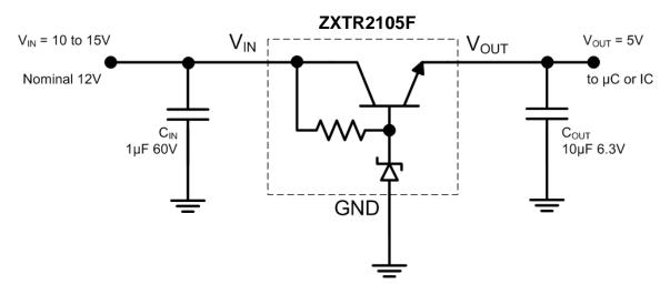
Example of a 5V regulated supply from a nominal 12V for powering a Controller IC.
