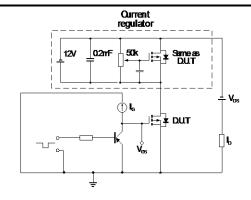
Gate charge test circuit
