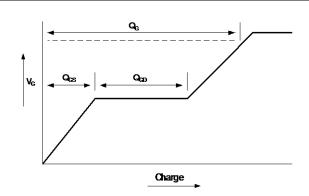
Basic gate charge waveform
