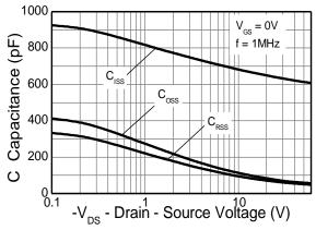
**Capacitance v Drain-Source Voltage**
