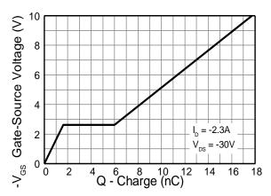
Gate-Source Voltage v Gate Charge
