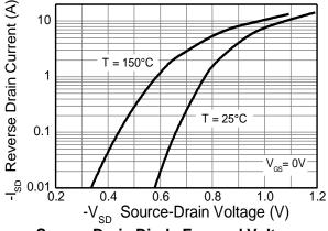
**Source-Drain Diode Forward Voltage**
