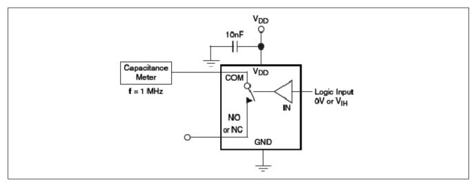
Figure 8. Channel On Capacitance
