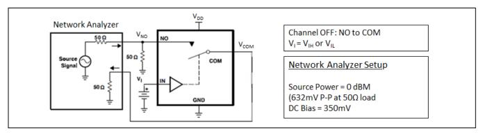
Figure 4. OFF Isolation (O<sub>ISO</sub>)
