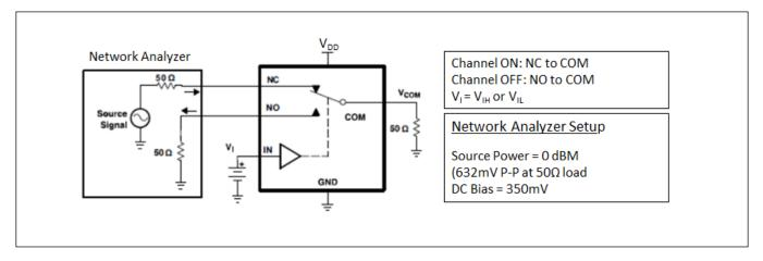
Figure 5. Channel-to-Channel Crosstalk
