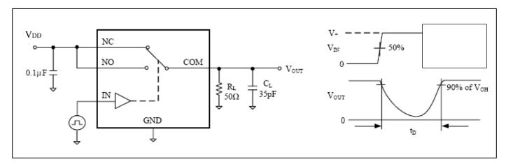
Figure 3. Break Before Make Interval Timing
