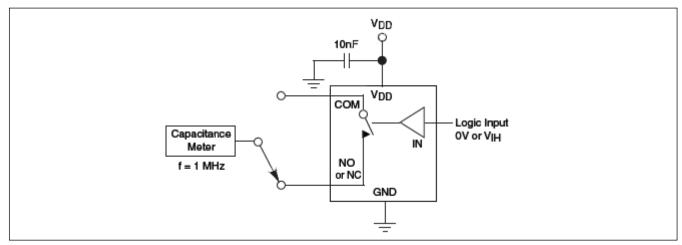
Figure 7. Channel Off Capacitance
