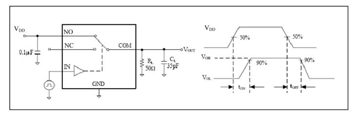
Figure 2. Switching Times
