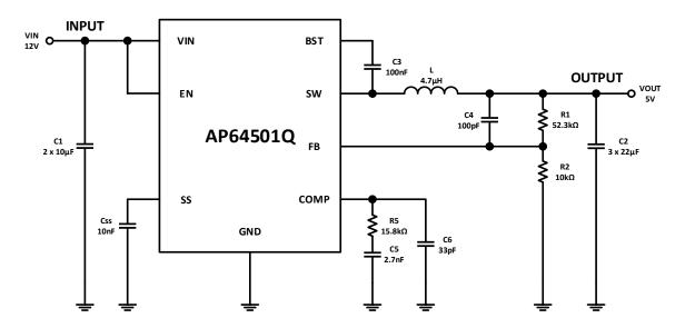
Figure 30. Example Circuit with Calculated Component Values for Loop Compensation
