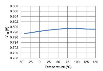
Figure 8. Feedback Voltage vs. Temperature, IOUT = 1A
