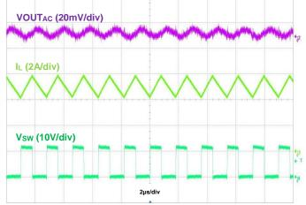
Figure 14. Output Voltage Ripple, VOUT = 5V, IOUT = 50mA
