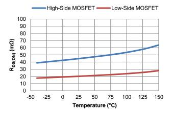
Figure 9. Power MOSFET RDS(ON) vs. Temperature
