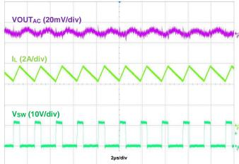
Figure 16. Output Voltage Ripple, VOUT = 3.3V, IOUT = 50mA
