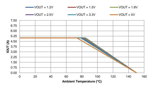
Figure 26. Output Current Derating Curve vs. Ambient Temperature, VIN = 12V
