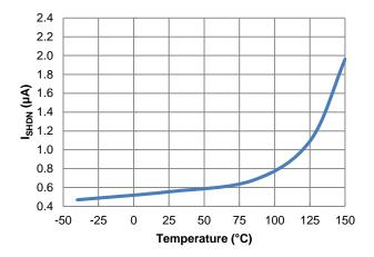
Figure 10. IQ vs. Temperature
