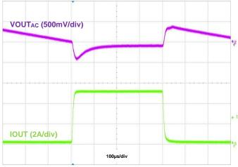
Figure 20. Load Transient, IOUT = 50mA to 5A to 50mA
