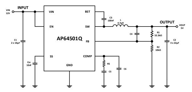
Figure 29. Example Circuit for Loop Compensation Calculations
