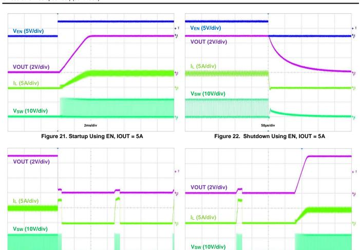
Figure 23. Output Short Protection, IOUT = 5A
