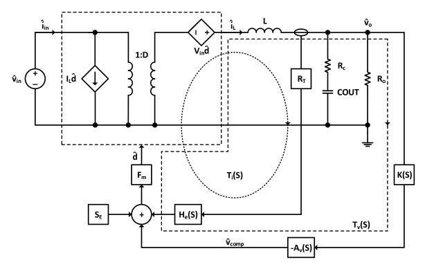
Figure 27. Small Signal Model of Buck Regulator
