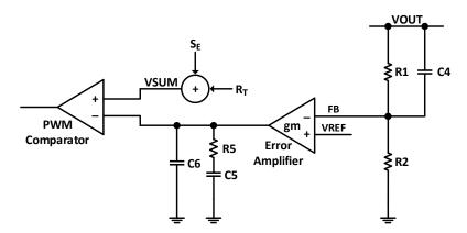
Figure 28. Type II Compensator
