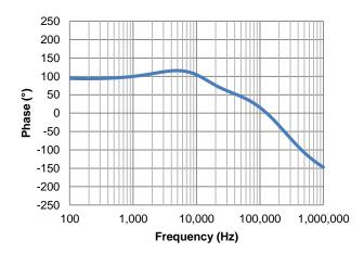
Figure 32. Closed-Loop Phase Margin
