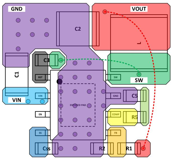
Figure 33. Recommended PCB Layout
