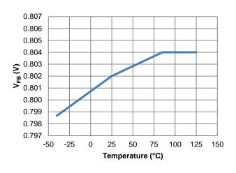
Figure 8. Feedback Voltage vs. Temperature
