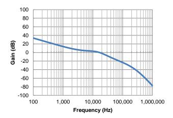
Figure 29. Closed-Loop Bandwidth
