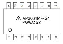
First Line: Logo and Marking ID Second Line: Date Code Y: Year WW: Work Week of Molding A: Assembly House Code XX: 7<sup>th</sup> and 8<sup>th</sup> Digits of Batch Number
