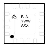
First Line: Logo and Marking ID Second Line: Date Code Y: Year WW: Work Week of Molding A: Assembly House Code XX: 7<sup>th</sup> and 8<sup>th</sup> Digits of Batch Number
