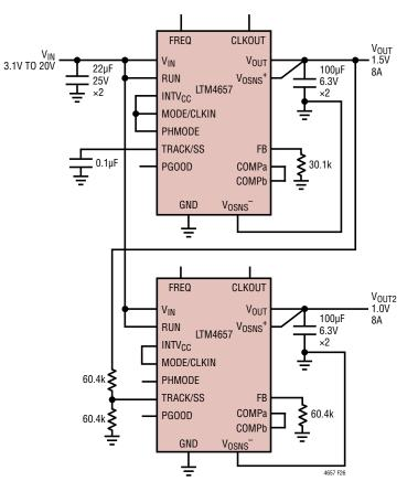
Figure 26. 3.1  $V_{\text{IN}}$  to  $20V_{\text{IN}},$  1.0V and 1.5V with Coincident Tracking
