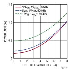
Figure 10. Power Loss at 1V Output
