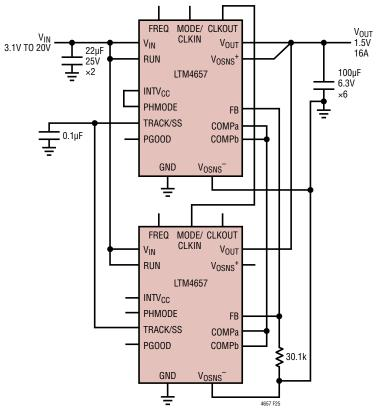
Figure 25. 3.1  $V_{\text{IN}}$  to  $20V_{\text{IN}},$  Two Phases, 1.5V at 16A Design
