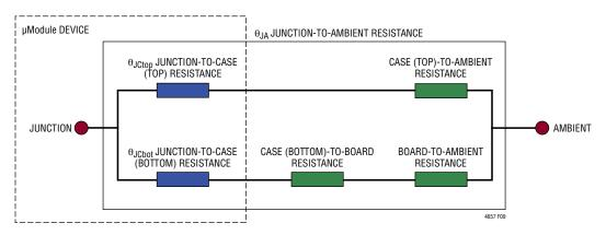
Figure 9. Graphical Approximation of the Thermal Coefficients, Including JESD 51-12 Terms
