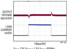
$\label{eq:VIN} \begin{array}{l} V_{IN} = 12V, \ V_{OUT} = 1.5V, \ f_{SW} = 650 \text{kHz}, \\ C_{OUT} = 2\times 100 \mu\text{F} + 22 \mu\text{F} \ \text{CERAMIC CAP}; \\ COMPa = COMPb \\ C_{FF} = 100 \mu\text{F} \end{array}$
