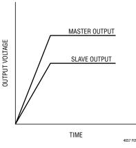
Figure 5. Output Ratiometric Tracking Waveform
