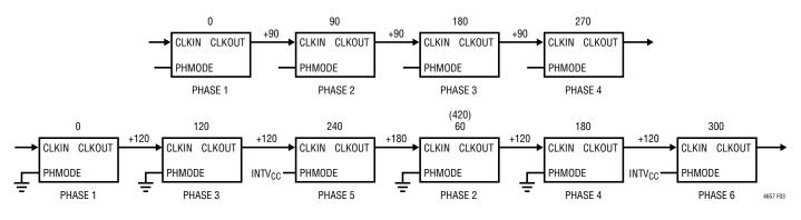
Figure 3. 4-Phase, 6-Phase Operation
