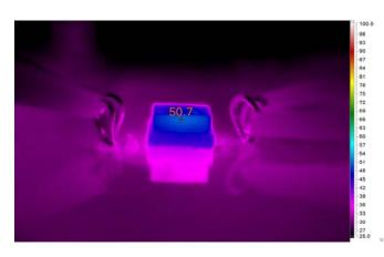
Figure 21. Thermal Image of LTM4657 Running from 12V Input and 1V Output at 8A Load at 25°C Ambient Without Airflow and Heat Sink
