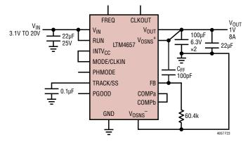
Figure 23. 3.1  $\rm V_{IN}$  to 20  $\rm V_{IN},$  1V Output at 8A Design
