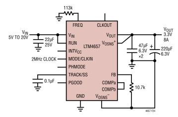
Figure 24.  $5V_{\text{IN}}$  to  $20V_{\text{IN}},$  3.3V Output with 2MHz External Clock
