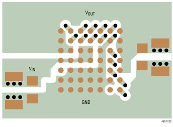
Figure 22. Recommended PCB Layout
