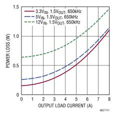
Figure 11. Power Loss at 1.5V Output
