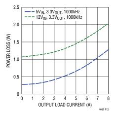
Figure 12. Power Loss at 3.3V Output
