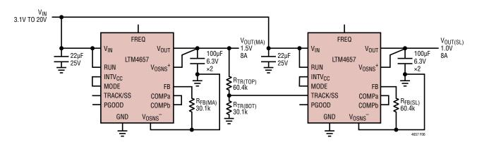
Figure 6. Example Schematic of Ratiometric Output Voltage Tracking
