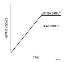
Figure 7. Output Coincident Tracking Waveform
