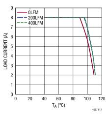
Figure 17. 12V to 1.5V Derating Curve, No Heat Sink
