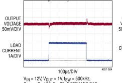
$\begin{array}{l} V_{IN}=12V,\,V_{OUT}=1V,\,f_{SW}=500kHz,\\ C_{OUT}=2\times100\mu F+22\mu F\,CERAMIC\,CAP;\\ COMPa=COMPb\\ C_{FF}=100pF \end{array}$
