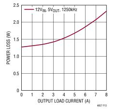
Figure 13. Power Loss at 5V Output
