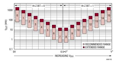
Figure 2. Frequency Range and Hi-Z Bit vs DIVCODE
