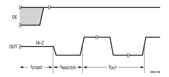
Figure 8. Start-Up Timing Diagram (OE = 1,  $N_{DIV} \geq 4, \; \text{Hi-Z} = 0 \; \text{or} \; 1)$
