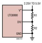
Figure 1. Simple Technique for Setting DIVCODE
