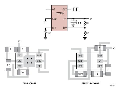
Figure 17. Supply Bypassing and PCB Layout
