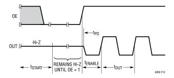
Figure 10. Start-Up Timing Diagram (OE = 0, N<sub>DIV</sub> = Any, Hi-Z = 1)
