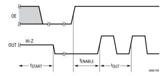
Figure 9. Start-Up Timing Diagram (OE = 0, N<sub>DIV</sub> = Any, Hi-Z = 0)
