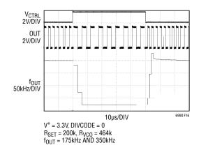
Figure 16. Settling Time
