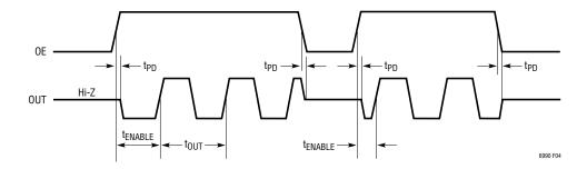
Figure 4. OE Timing Diagram (Hi-Z = 1)
