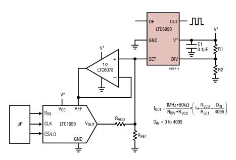
Figure 14. Digitally Controlled Oscillator with V<sub>SET</sub> Variation Eliminated
