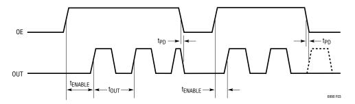
Figure 3. OE Timing Diagram (Hi-Z = 0)
