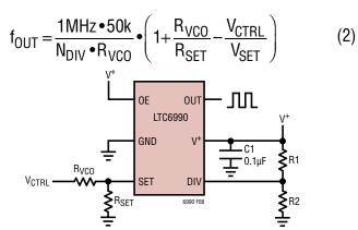
Figure 11. Voltage Controlled Oscillator
