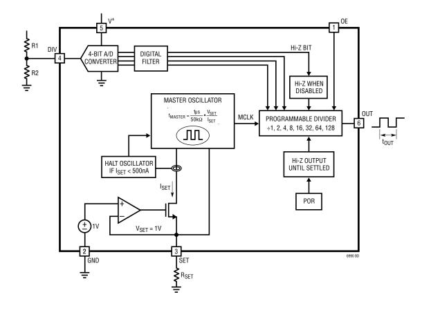
The LTC6990 is built around a master oscillator with a 1MHz maximum frequency. The oscillator is controlled by the SET pin current ( $I_{SET}$ ) and voltage ( $V_{SET}$ ), with a 1MHz • 50k conversion factor that is accurate to ±0.8% under typical conditions.
