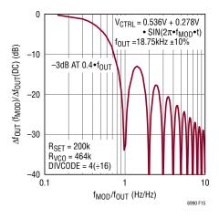
Figure 15. Modulation Frequency Response
