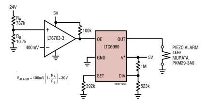
Direct Piezo Alarm Driver. Adjust Frequency for Maximum Alarm Sound Pressure (Maximum Annoyance for Best Effect)
