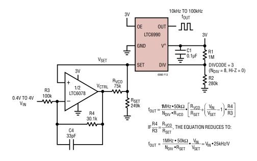
Figure 13. VCO with Reduced  $\Delta V_{SET}$  Sensitivity
