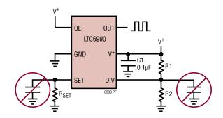
**OE** (**Pin 4/Pin 1**): Output Enable. Drive high to enable the output driver (Pin 6). Driving OE low disables the output asynchronously, so that the output is immediately forced low (Hi-Z = 0) or floated (Hi-Z = 1). When enabled, the output may temporarily remain low to synchronize with the internal oscillator in order to eliminate pulse slivers.
