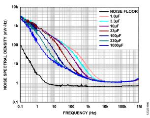
Figure 47. Noise Spectral Density vs. Frequency for Different Capacitances (C<sub>BYP</sub>)
