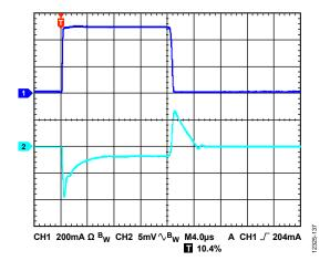
Figure 37. Load Transient Response,  $I_{LOAD}=10$  mA to 510 mA,  $V_{OUT}=1.8$  V,  $V_{IN}=2.3$  V, CH1 =  $I_{OUT}$ , CH2 =  $V_{OUT}$
