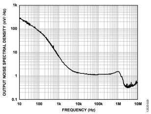
Figure 30. Output Noise Spectral Density, 10 Hz to 10 MHz, I<sub>LOAD</sub> = 100 mA
