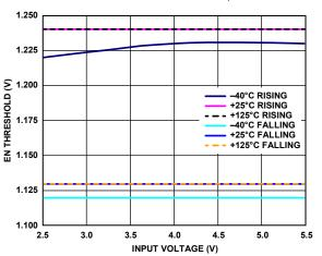
Figure 52. Typical EN Threshold vs. Input Voltages (V<sub>IN</sub>) for Different Temperatures
