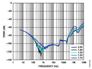
Figure 25. Power Supply Rejection Ratio (PSRR) vs. Frequency at Various Headroom Voltages,  $V_{\rm OUT} = 1.2 \, V$ , 400 mA Load
