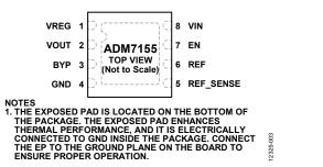
Figure 3. 8-Lead LFCSP Pin Configuration
