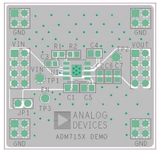
Figure 65. Example 8-Lead SOIC PCB Layout
