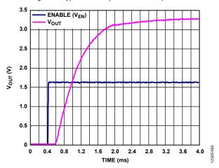
Figure 51. Typical  $V_{OUT}$  Response to EN Pin Operation ( $V_{EN}$ ),  $V_{OUT}=3.3~V$ ,  $V_{IN}=5~V$ ,  $C_{BYP}=1~\mu F$
