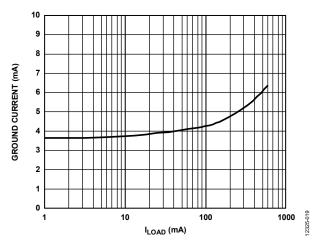
Figure 19. Ground Current vs. Load Current (ILOAD), VOUT = 1.2 V
