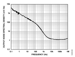
Figure 31. Output Noise Spectral Density, 0.1 Hz to 1 MHz, I<sub>LOAD</sub> = 10 mA
