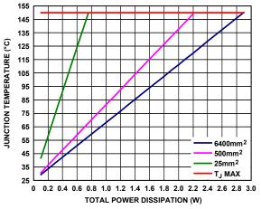
Figure 56. Junction Temperature vs. Total Power Dissipation for the 8-Lead LFCSP,  $T_A = 25^{\circ}\text{C}$
