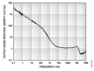
Figure 32. Output Noise Spectral Density, 0.1 Hz to 10 MHz,  $I_{LOAD} = 100$  mA
