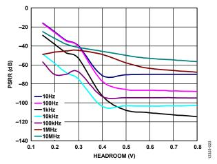
Figure 23. Power Supply Rejection Ratio (PSRR) vs. Headroom Voltage at Different Frequencies, Vout = 3.3 V, 400 mA Load
