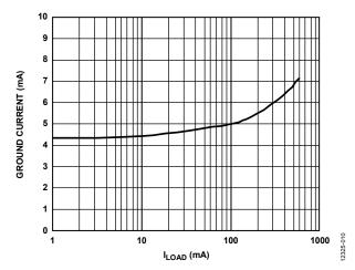
Figure 10. Ground Current vs. Load Current (ILOAD), VOUT = 3.3 V
