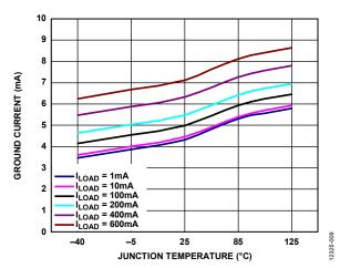
Figure 9. Ground Current vs. Junction Temperature (T,j) at Various Loads,  $V_{OUT} = 3.3~V$
