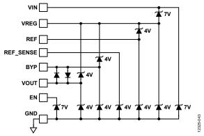
Figure 44. Simplified ESD Protection Block Diagram
