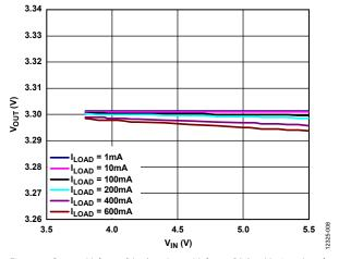
Figure 8. Output Voltage ( $V_{OUT}$ ) vs. Input Voltage ( $V_{IN}$ ) at Various Loads,  $V_{OUT} = 3.3~V$
