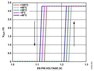
Figure 50. Typical V<sub>OUT</sub> Response to EN Pin Operation
