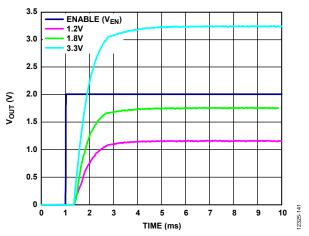
Figure 41.  $V_{\text{OUT}}$  Start-Up Time After  $V_{\text{EN}}$  Rising, Different Output Voltages,  $V_{\text{IN}} = 5 \text{ V}$
