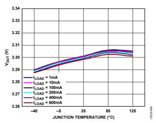
Figure 6. Output Voltage ( $V_{OUT}$ ) vs. Junction Temperature ( $T_J$ ) at Various Loads,  $V_{OUT}$  = 3.3 V
