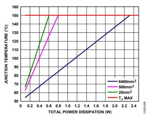
Figure 57. Junction Temperature vs. Total Power Dissipation for the 8-Lead LFCSP,  $T_A = 50^{\circ}C$
