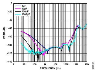
Figure 27. Power Supply Rejection Ratio (PSRR) vs. Frequency, Different  $C_{BYP}$ ,  $V_{OUT} = 3.3 V$ , 400 mA Load, 500 mV Headroom
