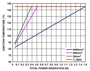
Figure 58. Junction Temperature vs. Total Power Dissipation for the 8-Lead LFCSP,  $T_A = 85^{\circ}C$
