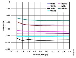
Figure 26. Power Supply Rejection Ratio (PSRR) vs. Headroom Voltage, Different Frequencies, V<sub>OUT</sub> = 1.2 V, 400 mA Load
