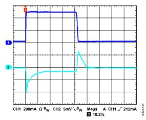
Figure 45. Output Transient Response,  $V_{OUT}$  = 3.3 V,  $C_{OUT}$  = 10  $\mu$ F, CH1 = Load Current, CH2 =  $V_{OUT}$
