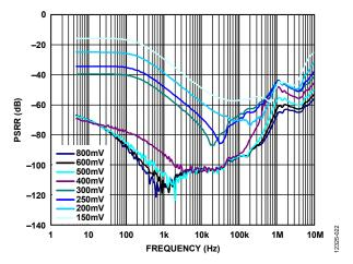
Figure 22. Power Supply Rejection Ratio (PSRR) vs. Frequency at Various Headroom Voltages,  $V_{OUT} = 3.3 V$ , 400 mA Load
