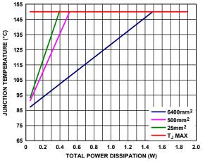
Figure 61. Junction Temperature vs. Total Power Dissipation for the 8-Lead SOIC,  $T_A = 85^{\circ}C$
