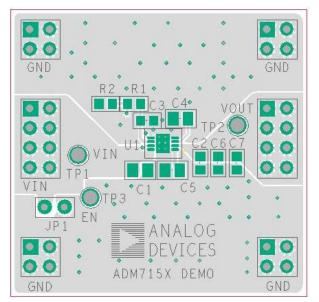
Figure 64. Example 8-Lead LFCSP PCB Layout
