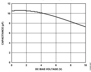
Figure 48. Capacitance vs. DC Bias Voltage
