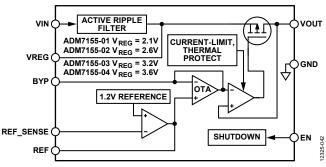
Figure 42. Simplified Internal Block Diagram
