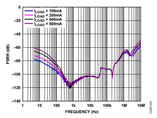
Figure 24. Power Supply Rejection Ratio (PSRR) vs. Frequency at Various Loads,  $V_{\text{OUT}} = 1.2 \text{ V}$ ,  $V_{\text{IN}} = 2.4 \text{ V}$
