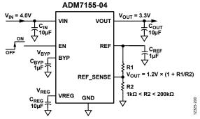
Figure 43. Typical Adjustable Output Voltage Application Schematic
