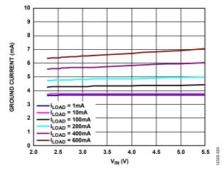
Figure 20. Ground Current vs. Input Voltage ( $V_{\text{IN}}$ ) at Different Loads,  $V_{\text{OUT}} = 1.2 \text{ V}$
