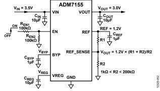
Figure 53. Typical EN Pin Voltage Divider
