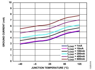
Figure 18. Ground Current vs. Junction Temperature (T<sub>J</sub>) at Various Loads,  $V_{OUT} = 1.2 V$
