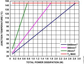
Figure 59. Junction Temperature vs. Total Power Dissipation for the 8-Lead SOIC,  $T_A = 25^{\circ}C$
