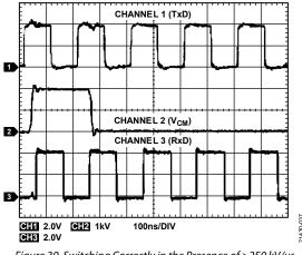
Figure 39. Switching Correctly in the Presence of >250 kV/µs Common-Mode Transients
