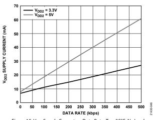
Figure 15.  $V_{DD2}$  Supply Current vs. Data Rate,  $T_A = 25^{\circ}$ C, No Load
