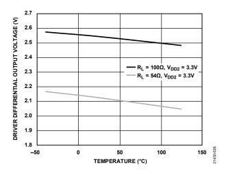
Figure 19. Driver Differential Output Voltage vs. Temperature
