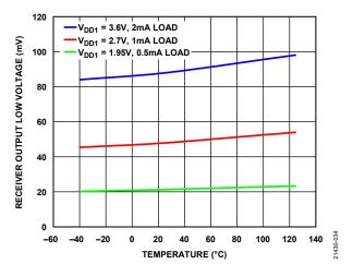
Figure 28. Receiver Output Low Voltage vs. Temperature
