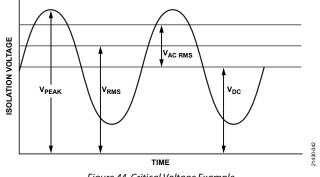
Figure 44. Critical Voltage Example
