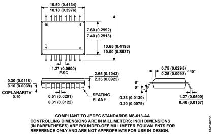
Figure 45. 16-Lead Standard Small Outline Package [SOIC\_W] Wide Body (RW-16) Dimensions shown in millimeters and (inches)
