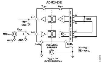
Figure 38. CMTI Test Diagram, Full Duplex
