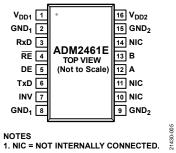
Figure 10. ADM2461E Half-Duplex Pin Configuration
