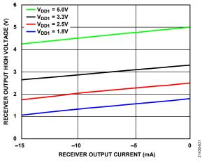
Figure 25. Receiver Output High Voltage vs. Receiver Output Current
