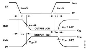
Figure 6. Receiver Enable or Disable Timing
