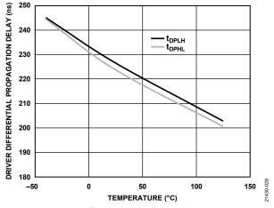
Figure 23. Driver Differential Propagation Delay vs. Temperature
