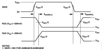
Figure 7. Receiver Cable Invert Timing Specification Measurement
