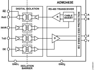
Figure 2. ADM2463E Functional Block Diagram
