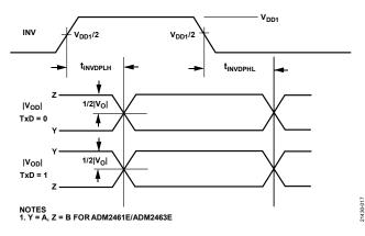
Figure 8. Driver Cable Invert Timing Specification Measurement
