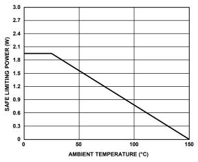
Figure 9. Thermal Derating Curve for 16-Lead, Standard, Wide Body SOIC\_W, Dependence of Safety Limiting Values with Ambient Temperature per DIN V VDE V 0884-10
