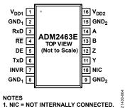
Figure 11. ADM2463E Full Duplex Pin Configuration
