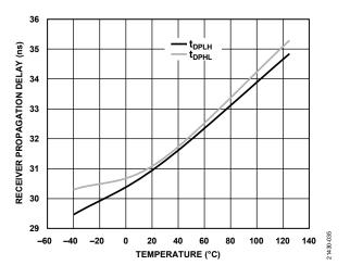
Figure 29. Receiver Propagation Delay vs. Temperature
