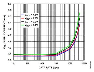
Figure 18. V<sub>DD1</sub> Supply Current vs. Data Rate
