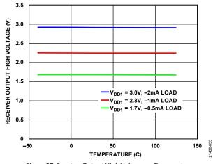
Figure 27. Receiver Output High Voltage vs. Temperature
