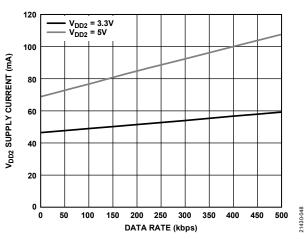
Figure 17.  $V_{DD2}$  Supply Current vs. Data Rate,  $T_A = 25$  °C,  $R_L = 54 \Omega$
