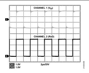
Figure 30. Receiver Switching at 500 kbps
