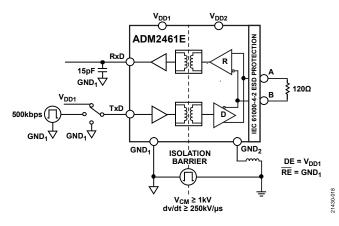
Figure 37. CMTI Test Diagram, Half-Duplex
