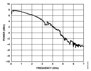
Figure 15. RF<sub>OUT</sub>A+/RF<sub>OUT</sub>A – Power vs. Frequency (100 nH Inductors, 100 pF Bypass Capacitors, Board Measurement)
