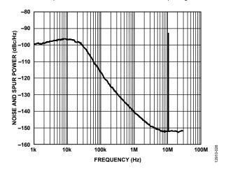
Figure 20. Fractional-N Spur Performance, RF<sub>OUT</sub>A+ = 2.591 GHz, REF<sub>IN</sub> = 122.88 MHz, PFD = 61.44 MHz, Output Divide-by-2 Selected, Loop Filter Bandwidth = 20 kHz, Channel Spacing = 20 kHz
