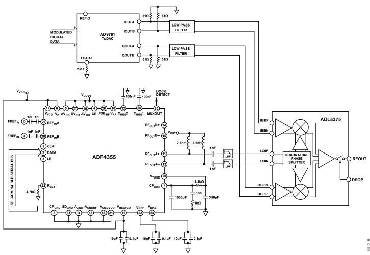
Figure 44. Direct Conversion Modulator
