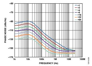
Figure 8. Closed-Loop Phase Noise, RF<sub>OUT</sub>A+, Fundamental VCO and Dividers, VCO = 5.0 GHz, PFD = 61.44 MHz, Loop Bandwidth = 20 kHz
