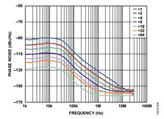
Figure 9. Closed-Loop Phase Noise, RF<sub>OUT</sub>A+, Fundamental VCO and Dividers, VCO = 6.8 GHz, PFD = 61.44 MHz, Loop Bandwidth = 20 kHz
