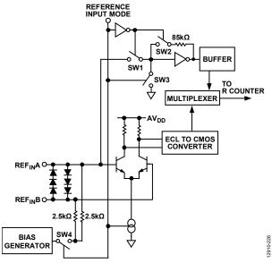
Figure 22. Reference Input Stage
