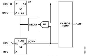
Figure 24. PFD Simplified Schematic
