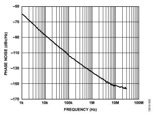
Figure 5. Open-Loop VCO Phase Noise, 5.0 GHz
