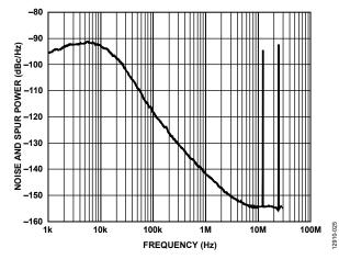
Figure 19. Fractional-N Spur Performance, W-CDMA Band,  $RF_{OUT}A+=2113.5$  MHz,  $REF_{IN}=122.88$  MHz, PFD=61.44 MHz, Output Divide by 2 Selected, Loop Filter Bandwidth = 20 kHz, Channel Spacing = 20 kHz
