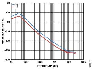
Figure 11. Closed-Loop Phase Noise, RF<sub>OUT</sub>A+, Fundamental VCO and Divide by 2, VCO = 5.0 GHz, PFD = 61.44 MHz, Loop Bandwidth = 2 kHz
