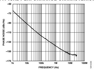
Figure 4. Open-Loop VCO Phase Noise, 3.4 GHz
