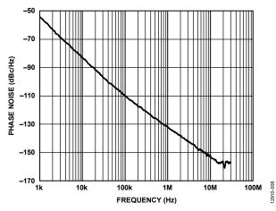
Figure 6. Open-Loop VCO Phase Noise, 6.8 GHz
