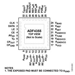
Figure 3. Pin Configuration
