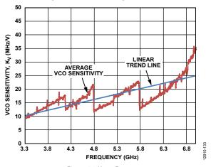
Figure 26. K<sub>V</sub> vs. Frequency
