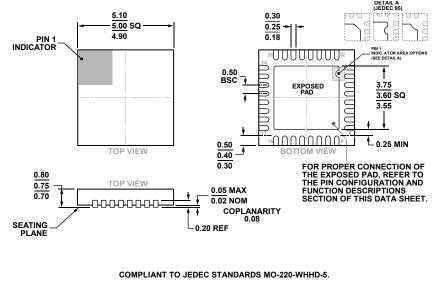
Figure 47. 32-Lead Lead Frame Chip Scale Package [LFCSP] 5 mm × 5 mm Body and 0.75 mm Package Height (CP-32-12) Dimensions shown in millimeters
