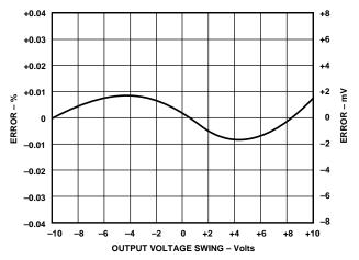
Figure 12. Gain Nonlinearity Error vs. Output
