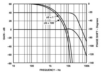
Figure 10. Phase Shift and Gain vs. Frequency
