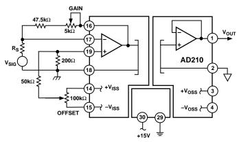
Figure 6. Adjustments for Inverting Input
