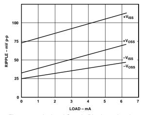
Figure 16a. Isolated Supply Ripple vs. Load (External 4.7 µF Bypass)
