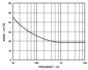
Figure 11. Input Noise vs. Frequency
