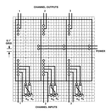
Figure 8. PCB Layout for Multichannel Applications with Gain
