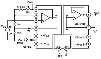
Figure 5. Adjustments for Noninverting Input
