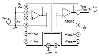
Figure 3. Input Configuration for G > 1
