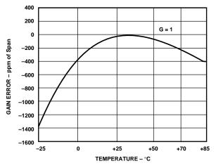
Figure 14. Gain vs. Temperature
