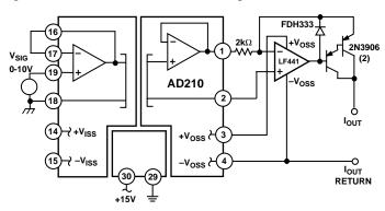
Figure 18. Self-Powered Isolated Current Source
