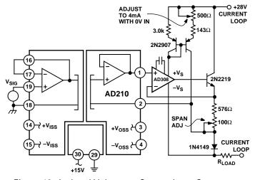
Figure 19. Isolated Voltage-to-Current Loop Converter
