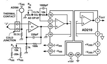
Figure 20. Isolated Thermocouple Amplifier
