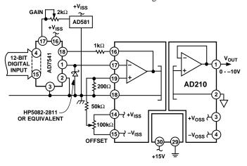
Figure 21. Precision Floating Programmable Reference
