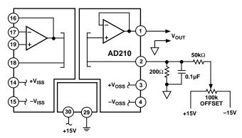
Figure 7. Output-Side Offset Adjustment
