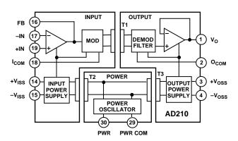
mode voltage isolation between any two ports. Low input capacitance of 5 pF results in a 120 dB CMR at a gain of 100, and a low leakage current (2 µA rms max @ 240 V rms, 60 Hz).
