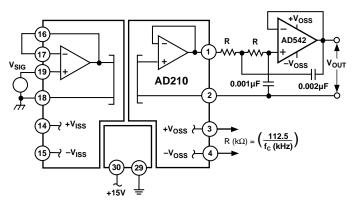
Figure 17. 2-Pole, Output Filter
