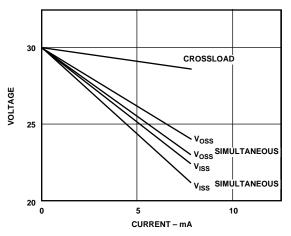
Figure 15. Isolated Power Supplies vs. Load
