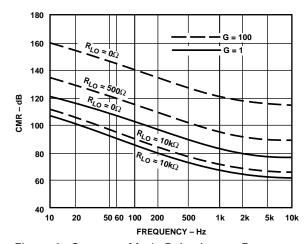
Figure 9. Common-Mode Rejection vs. Frequency
