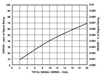
Figure 13. Gain Nonlinearity vs. Output Swing
