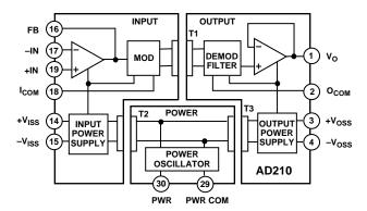
Figure 1. AD210 Block Diagram
