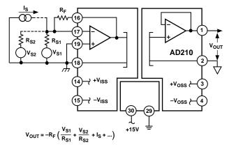
Figure 4. Summing or Current Input Configuration
