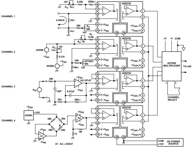
Figure 22. Multichannel Data Acquisition Front-End
