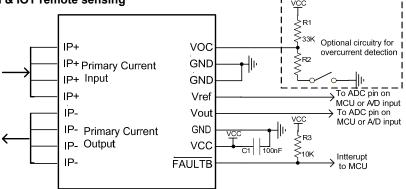
Figure 1 - Application circuit
