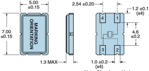
Note: Chamfer and index mark not shown.
