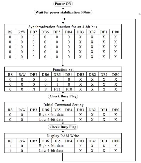
Note: Initial code is for reference only. Please make the best adjustment with the OLED module.
