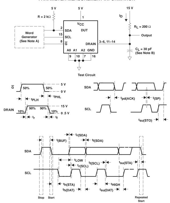
NOTES: A. The word generator has the following characteristics:  $t_r \le 30$  ns,  $t_f \le 30$  ns, pulsed repetition rate (PRR) = 400 kHz,  $Z_O = 50 \ \Omega$ .
