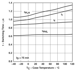
Figure 6. Switching Time vs Case Temperature
