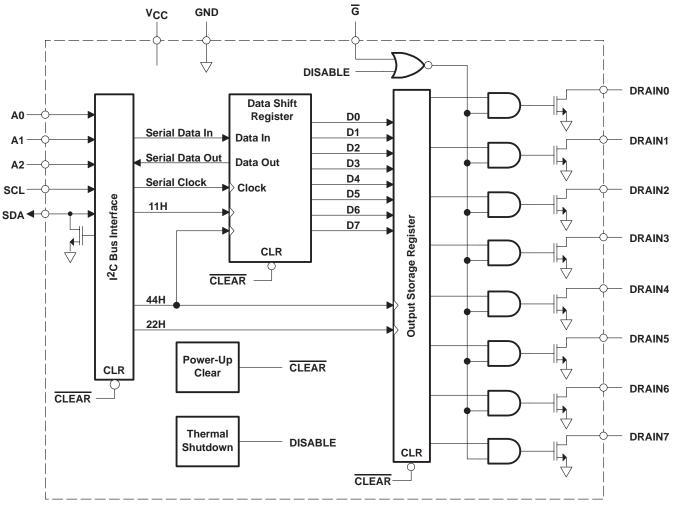
See the *TPIC2810* subaddress and *I*<sup>2</sup>C protocol definition section of this data sheet for definition of the 11H, 22H, and 44H control signals.
