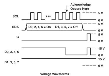
NOTES: A. The word generator has the following characteristics:  $t_r \le 30$  ns,  $t_f \le 30$  ns, pulsed repetition rate (PRR) = 400 kHz,  $Z_O = 50 \ \Omega$ .
