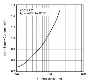
Figure 3. Supply Current vs Frequency
