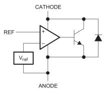
Figure 21. Equivalent Schematic
