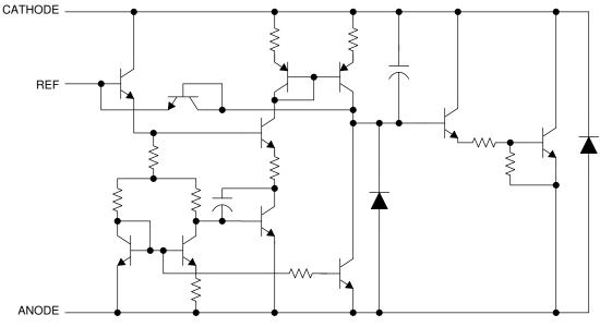
Figure 22. Detailed Schematic
