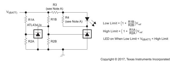
A. Select R3 and R4 to provide the desired LED intensity and cathode current  $\ge$  0.08 mA to the ATL431LI at the available V<sub>I(BATT)</sub>.
