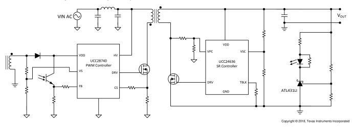
Figure 28. Isolated Flyback with Optocoupler
