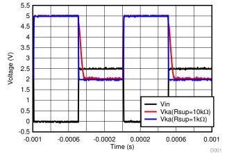
Figure 24. Output Response With Various Cathode Currents
