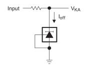
Figure 19. Test Circuit for I<sub>off</sub>
