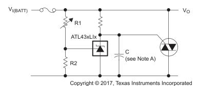
A. Refer to the stability boundary conditions in and Figure 13 to determine allowable values for C.
