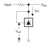
Figure 17. Test Circuit for  $V_{KA} = V_{ref}$
