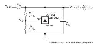
Figure 26. Shunt Regulator Schematic
