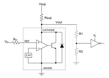
Figure 23. Comparator Application Schematic
