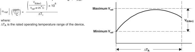
$\alpha_{Vref}$  is positive or negative, depending on whether minimum V<sub>ref</sub> or maximum V<sub>ref</sub>, respectively, occurs at the lower temperature. The full-range temperature coefficient is an average and therefore any subsection of the rated operating temperature range can yield a value that is greater or less than the average. For more details on temperature coefficient, check out *Voltage Reference Selection Basics*.
