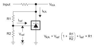
Figure 18. Test Circuit for  $V_{KA} > V_{ref}$
