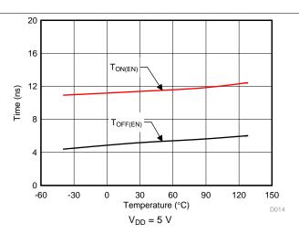
Figure 14. T<sub>ON (EN)</sub> and T<sub>OFF (EN)</sub> vs Temperature
