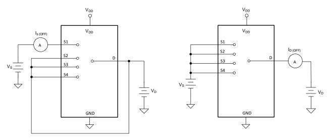
Figure 19. Off-Leakage Measurement Setup
