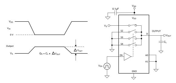
Figure 24. Charge-Injection Measurement Setup
