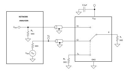
Figure 26. Crosstalk Measurement Setup
