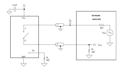
Figure 25. Off Isolation Measurement Setup
