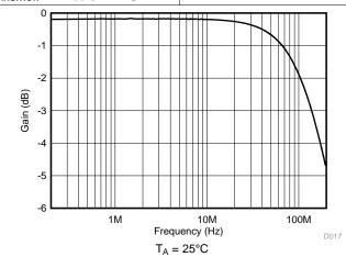
Figure 17. On Response vs Frequency
