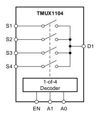
Figure 28. TMUX1104 Functional Block Diagram
