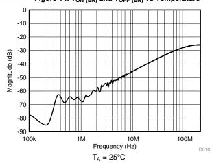
Figure 16. Xtalk and Off-Isolation vs Frequency
