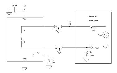
Figure 27. Bandwidth Measurement Setup
