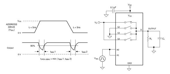
Figure 22. Break-Before-Make Delay Measurement Setup
