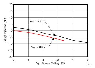
Figure 31. Charge Injection vs Source Voltage
