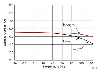
Figure 29. Leakage Current vs Temperature
