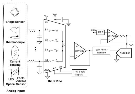
Figure 32. Multiplexing Signals to External ADC
