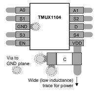
Figure 35. TMUX1104 Layout Example
