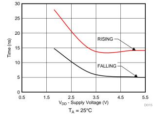
Figure 15. Output T<sub>TRANSITION</sub> vs Supply Voltage
