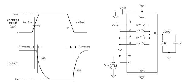
Figure 21. Transition-Time Measurement Setup
