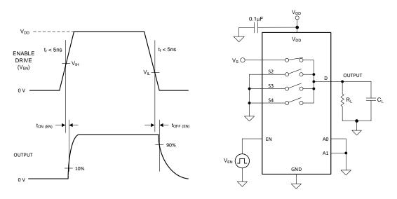
Figure 23. Turn-On and Turn-Off Time Measurement Setup
