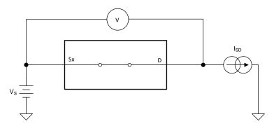
Figure 18. On-Resistance Measurement Setup
