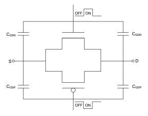
Figure 30. Transmission Gate Topology
