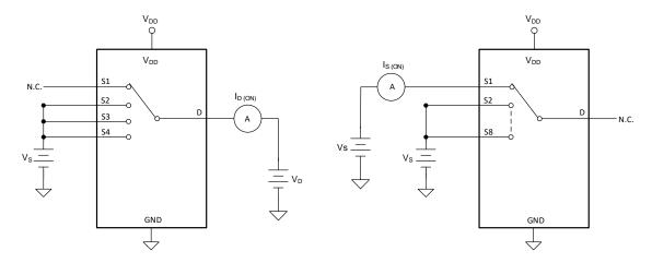
Figure 20. On-Leakage Measurement Setup
