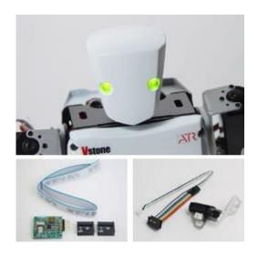
And its UI design is pretty nice. Each sturdy aluminum frame has screw holes for easy parts location and assembly. By knowing the structure well, you can jump over to remodel and modify it. Besides, the Vstone team has developed the full-featured controlling software "RobovieMaker", which is already packed for your dashboard. With a cool gear, a PS2 gamepad that Robovie-X supports, you are ready to go and have fun in real-life game.
