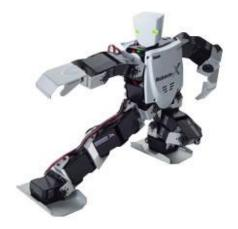
All these features are empowered by its luxurious configuration. Seventeen VS-S092J servos with up to 9.2kg/cm torque provide reliable seventeen degrees of freedom. A built-in audio system on the onboard controller and LED blinking eyes allow it to reflect its moods and interact with you. Have a brilliant idea to add a
