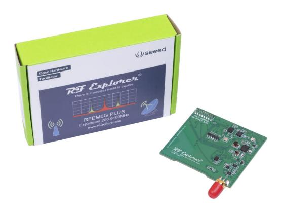
RF Explorer RFEM6G PLUS is an expansion module to convert a RF Explorer WSUB1G PLUS into a powerful 6G Combo PLUS Spectrum Analyzer, covering the full range starting at 50KHz up to 6.1GHz with no gaps or limitations.
